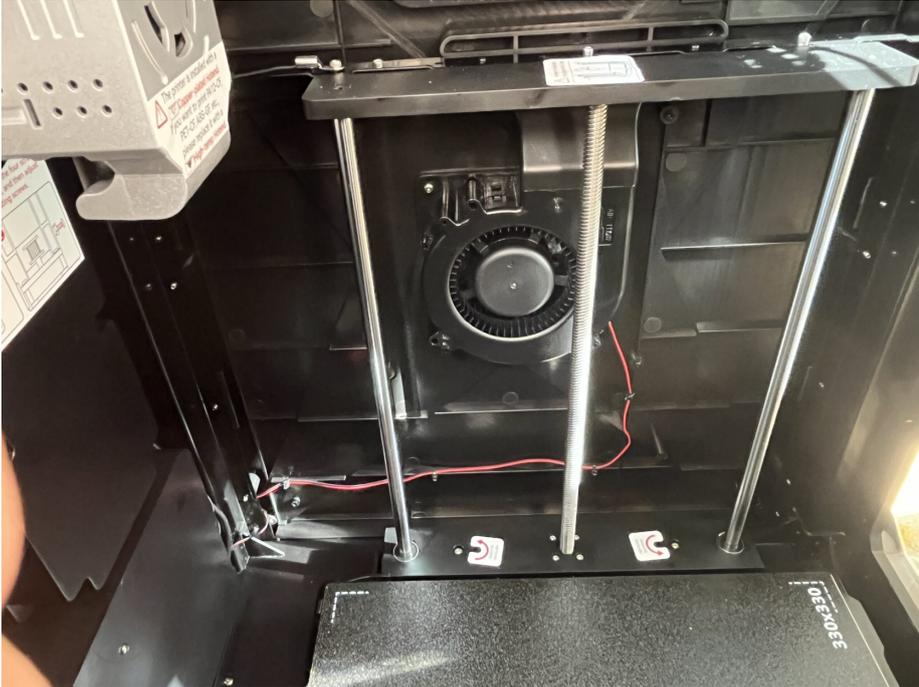
(Rods and leadscrew on one side. Picture by <https://drucktipps3d.de/qidi-x-max-3-testbericht/> )
